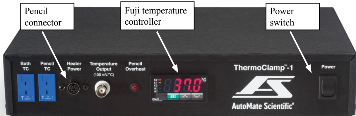
Figure 1. Controller unit, front view. (TC = thermocouple temperature sensor)
