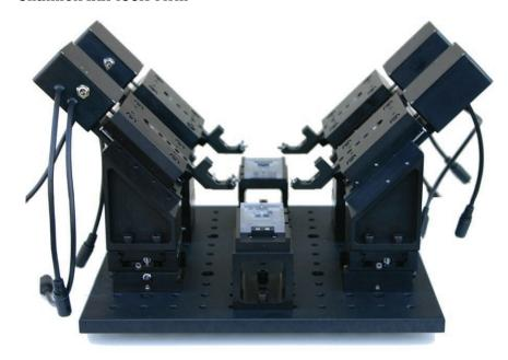
This system is similar to the ChannelMAX 100A Mini except it can be used for doing two two-electrode voltage clamp experiments or up to four patch clamp experiments simultaneously.
