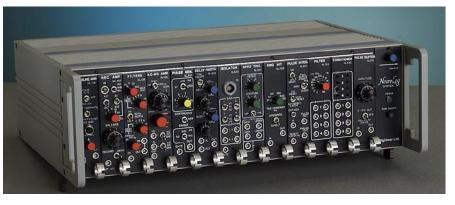
be installed. This means that a single NeuroLog System can be used to amplify several different parameters, such as extracellular spikes, intracellular potentials or even blood pressure, as well as produce outgoing trigger pulses to other pieces of equipment or electrically stimulate a preparation.
