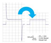
The patented Spread Frequency Compensation can automatically compensate any arbitrary capacitance profile in approximately 3 seconds.
