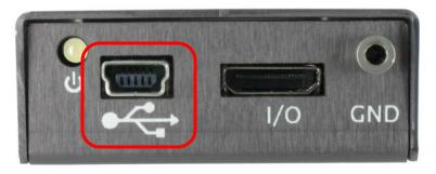
When plugging in the Pico for the first time, the driver will automatically be installed. Follow the on-screen instructions to install the Pico driver.
