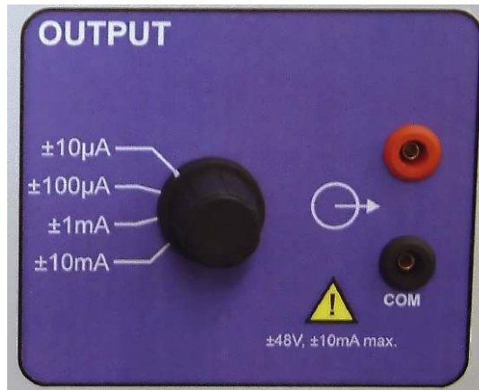
Figure 6 The OUTPUT zone of the DS4 front panel.
