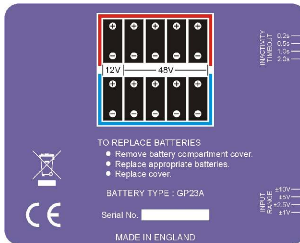
Figure 12 DS4 battery compartment labelling.
