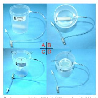
ABOVE: Components of BSK1 slice keeper and Holder BSKV: A BSKV consists of a 200ml trough fitted with a ceramic air stone and needle valve regulator for fine control of gas. B View of BSKV from above. C BSKV with BSK1 in place and D viewed from above. BELOW: Dimensions
